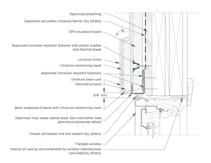
NOTE 1: Maintain 1/8" space between beveled insulation and weep casing bead. NOTE 2: At horizontal wall surfaces, including ledges, caps, sills, etc. a minimum slope of 6" in 12" is required.
